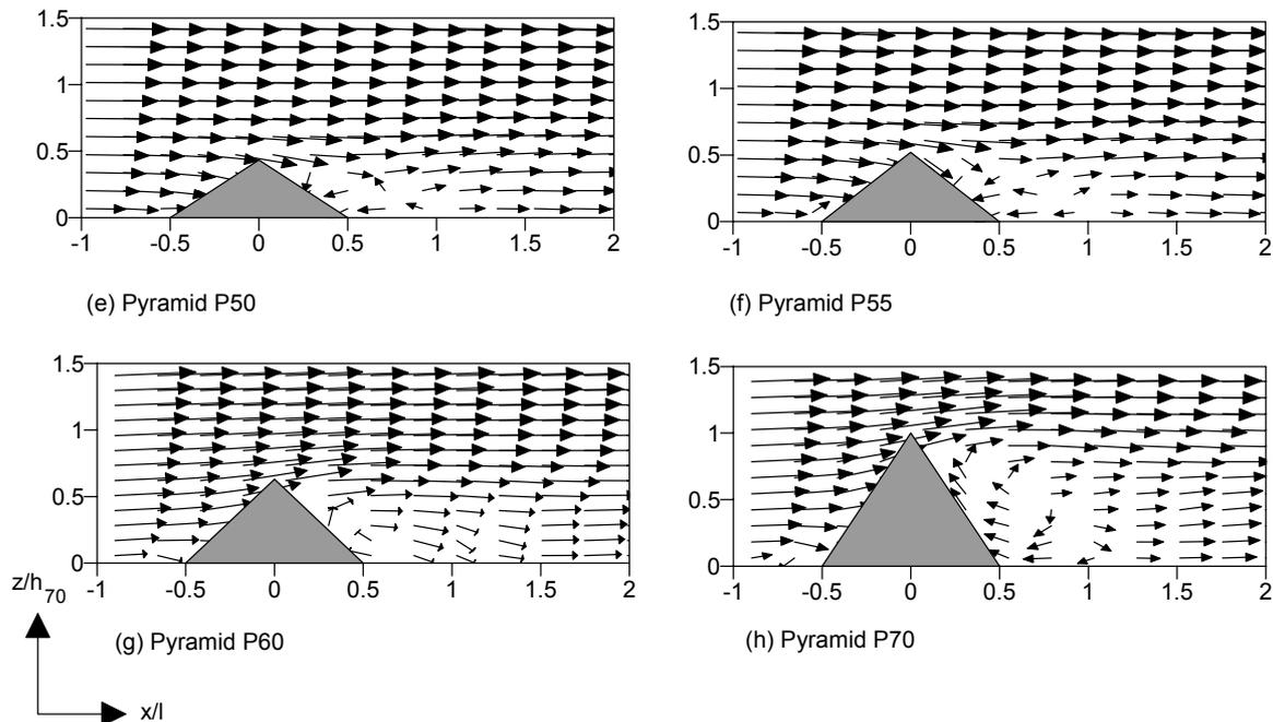
Figure 4 (e) – (h). Velocity vector fields at the center line cross section ( $y/l=0$ ) of pyramids ( $\alpha'=0^\circ$ ,  $u_\infty = 5$  m/s,  $h_{70} = 274.7$  mm)
