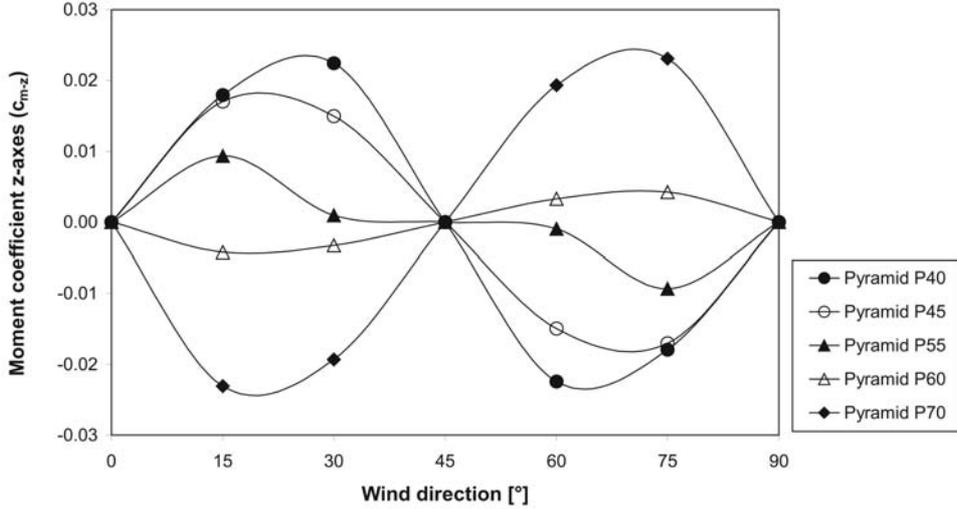
Figure 7(a). Moment coefficient ( $c_{m-z}$ ) as a function of wind direction
