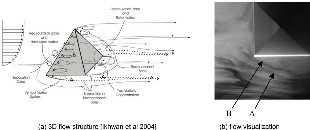
Figure 1. Flow structure around a pyramid
