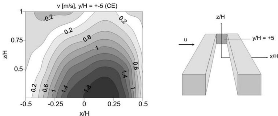
Figure 4. Mean horizontal velocity  $v$  at canyon ends ( $y/H = \pm 5$ ).
