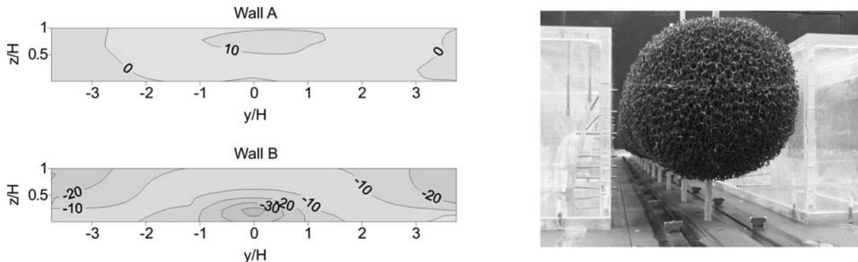
Figure 7. Relative change (%) in concentrations for street canyon with permeable tree crowns of 15 m crown diameter and 15 m spacing when compared to street canyon with impermeable tree crowns (Figure 5).
