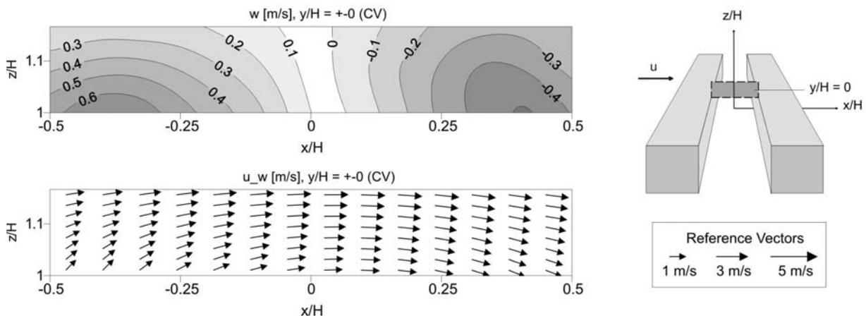
Figure 3. Velocity field at canyon center ( $y/H = 0$ ) in roof top level for reference case without trees.
