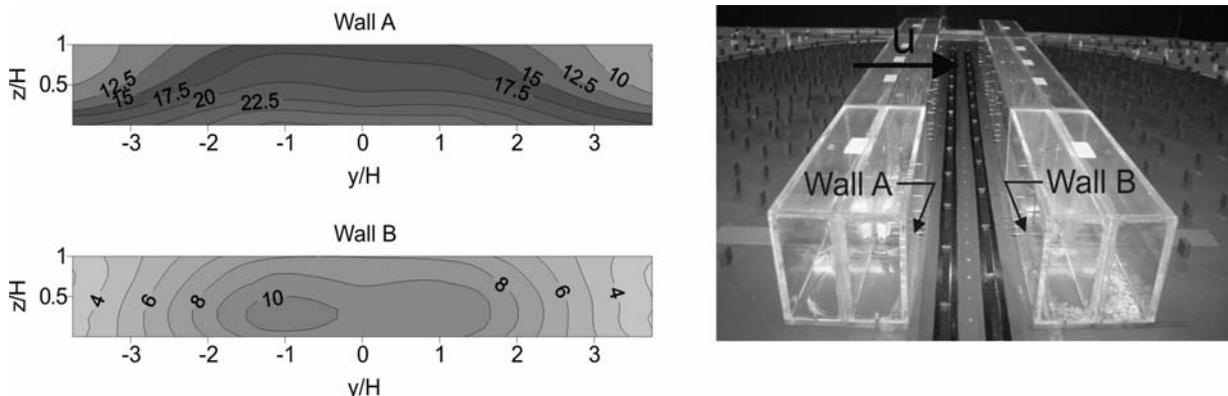
Figure 2. Dimensionless wall concentrations for reference case without trees.
