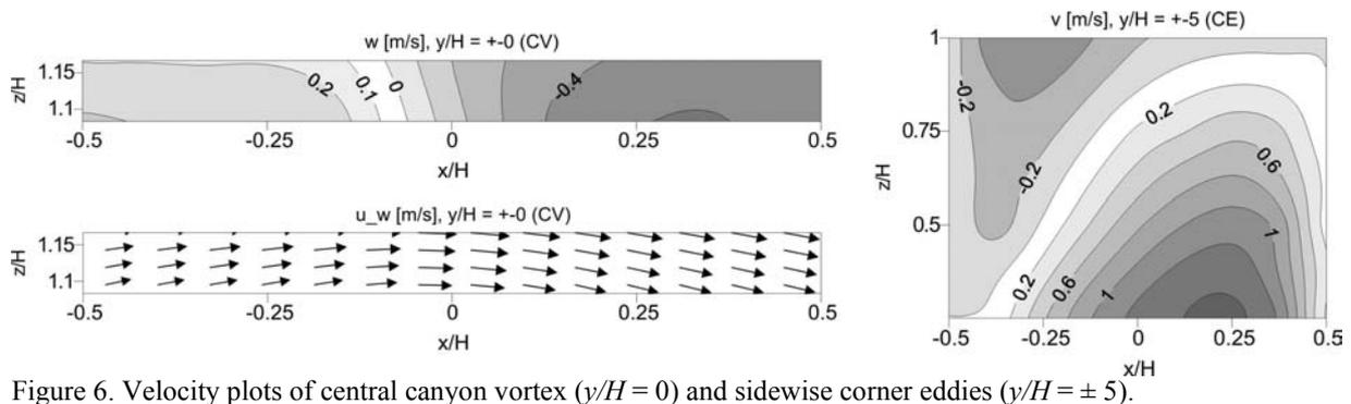
Figure 6. Velocity plots of central canyon vortex ( $y/H = 0$ ) and sidewise corner eddies ( $y/H = \pm 5$ ).
