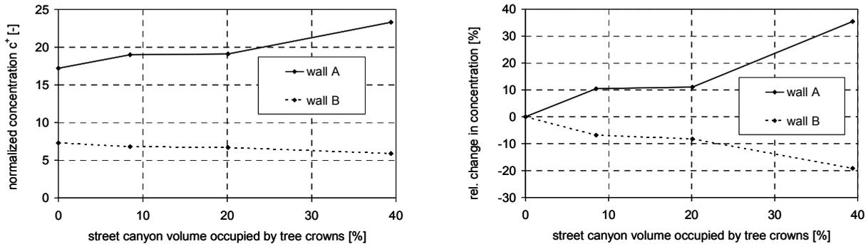
Figure 8. Wall averaged concentrations in dependency on street canyon volume occupied by tree crowns.
