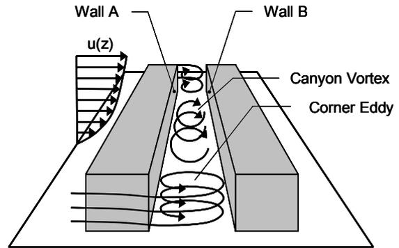
Figure 1. Model setup and flow field inside street canyon.
