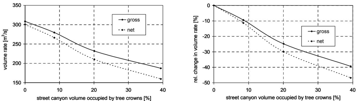
Figure 9. Volume rates of flow entering the street canyon horizontally through cross sections at  $y/H = \pm 5$  in dependency on street canyon volume occupied by tree crowns.
