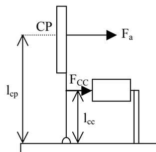
*Fig. 2 Sketch of the set-up employed to measure the drag force in the model.*
