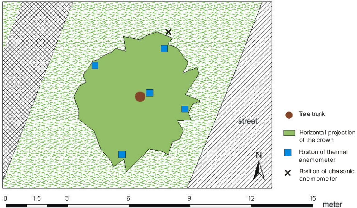
Figure 4: Measuring set-up the height above ground is 5.5 m, the sensor below the crown and the cup anemometer are not shown in this picture.
