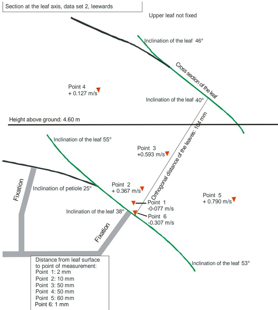
Figure 3: Measurement set-up for hot-wire anemometer measurements
